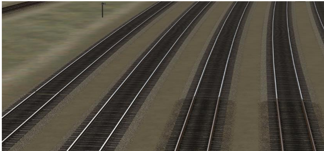
The singular track profile on this route looks great for the mainline (left) but is unsightly when used on the yard track (right).
